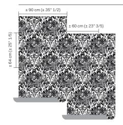
References A L U 2 Composition: rayon warps on non-woven backing Weight:  $\pm$  295 g/m² ( $\pm$  8,7 oz/sq yd) The wallcovering can be installed vertically or horizontally. Custom colouring on request.
